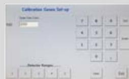
Use this page to set span gas concentrations. Users may set one concentration for each range on each measurement channel. Exit returns to Main screen.
