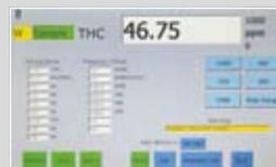
This gives channel specific details such as controlled temperatures, pressures and flows, and allows individual selection of controls for this specific channel, i.e. measurement modes (sample/zero/span/pause), calibration, abandon calibration, errors and choice of range or autorange. Exit takes you to Main screen.
