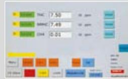
Shows up to 3 channels of information (error condition, measure state, gas type, concentration, range in use, unit in use). Has links to further detail for each channel. Buttons for menu and logging measure state (sample, zero, span, pause, standby and sleep), calibration, abandon calibration, whether to apply calibration to a single range or every range, alarm clearance and user logout. Also gives general analyser details (time/date/serial number/software versions/etc).
