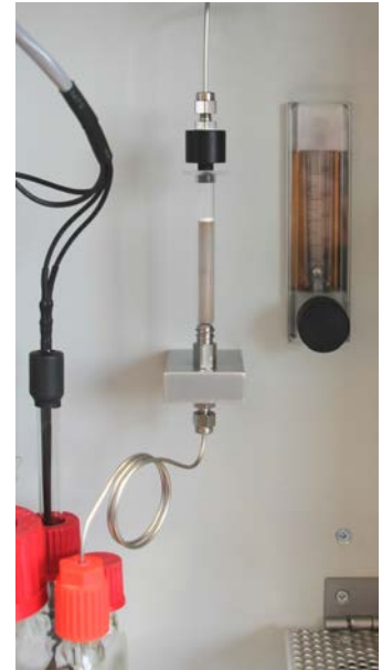
Sulphur trap for elimination of \text{H}_2\text{S} and mercaptans
